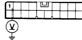
4WS CONTROL UNIT 18P CONNECTOR
